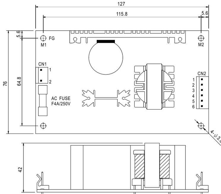
AC Input Connector (CN1) : Molex 5277-02 or equivalent
