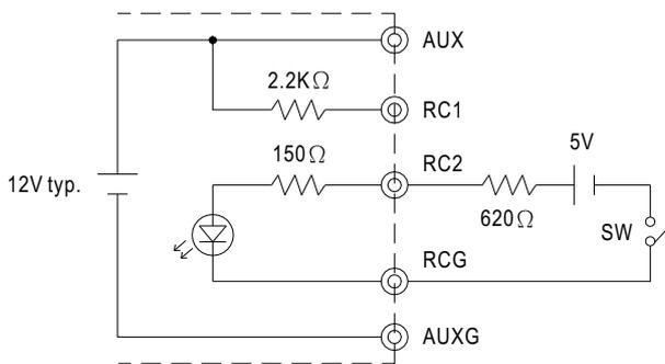
(B)Using internal 12V auxiliary output
